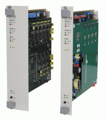
Figure 2. – ADSL Pair Gain CU
